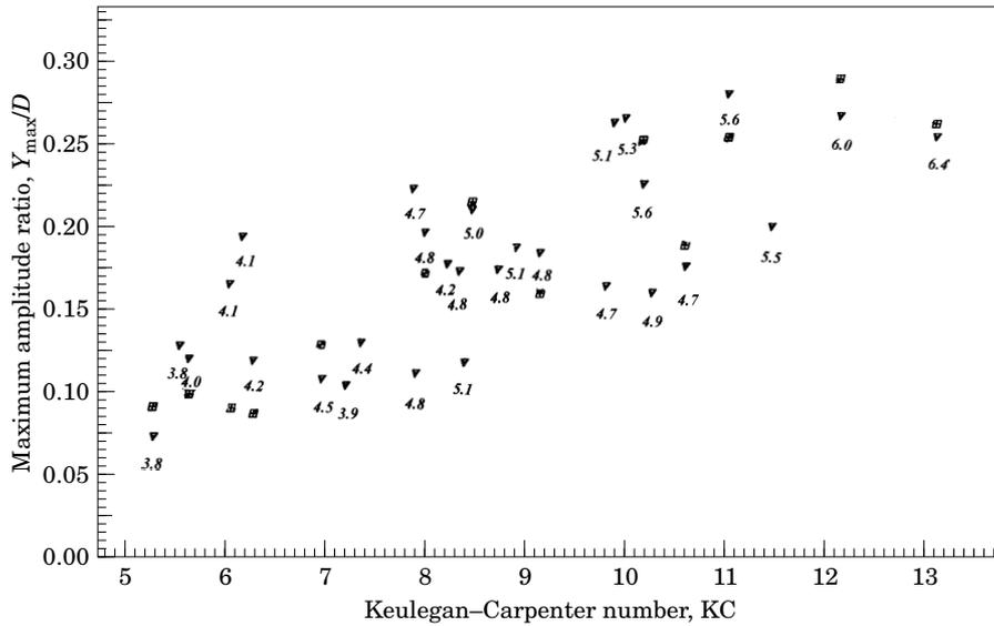
Figure 8. Results of the maximum transverse amplitude versus Keulegan-Carpenter number for various  $V_r$  values;  $D = 0.050$  m,  $G/D = 1$ ,  $K_s = 10.93$ . ( $\nabla$ ) Experiments; ( $\square$ ) predictions.
