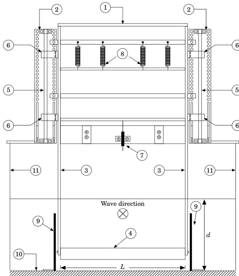
Figure 1. Schematic diagram of the test rig 2. ①—Frame 1; ②—Frame 2; ③—Aluminium bar; ④—Test cylinder; ⑤—Vertical shaft; ⑥—Linear ball bearings; ⑦—Potentiometer; ⑧—Springs; ⑨—End plates; ⑩—Bed of wave flume; ⑪—Walls of flume;  $d$ : Water depth;  $L$ : Cylinder length.
