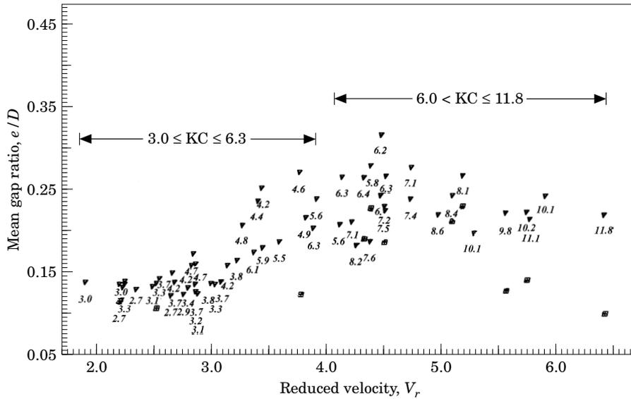
Figure 7. Results of the mean gap versus the reduced velocity for various  $Kc$  numbers;  $D = 0.060$  m,  $G/D = 0.126$ ,  $K_s = 10.30$ . ( $\nabla$ ) Experiments; ( $\square$ ) predictions.
