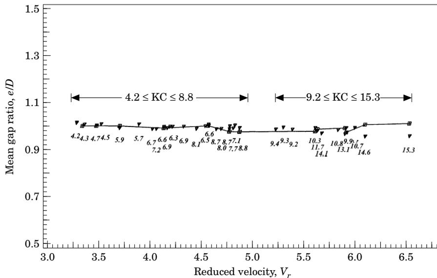
Figure 6. Results of the mean gap versus the reduced velocity for various  $KC$  numbers;  $D = 0.060$  m,  $G/D = 1$ ;  $K_s = 10-30$ . ( $\nabla$ ) Experiments; ( $\square$ ) predictions.
