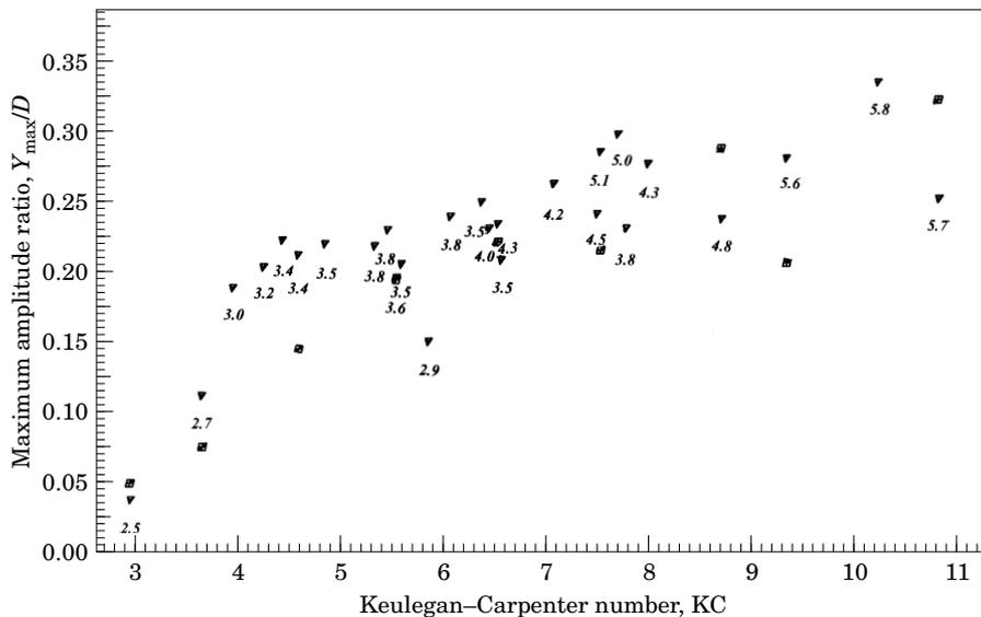
Figure 9. Results of the maximum transverse amplitude versus Keulegan-Carpenter number for various  $V_r$  values;  $D = 0.050$  m,  $G/D = 0.126$ ,  $K_s = 10.93$ . ( $\nabla$ ) Experiments; ( $\square$ ) predictions.
