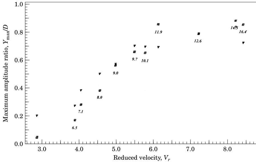
Figure 11. Results of the maximum transverse amplitude versus the reduced velocity for various KC numbers: (∇) experimental data of Anand & Torum (1985); (□) present numerical predictions;  $D = 0.050$  m,  $G/D = 1$ ,  $K_s = 0.180$ .
