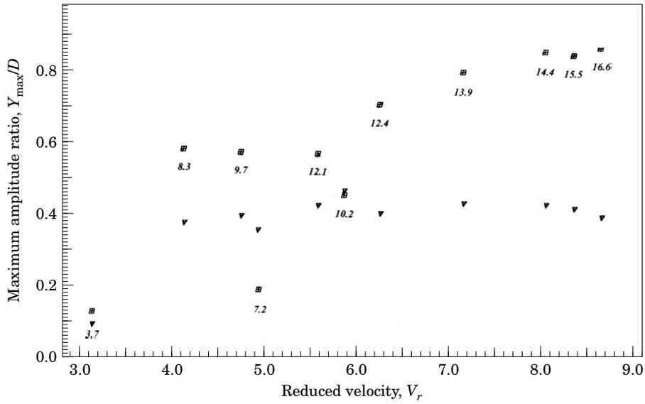
Figure 12. Results of the maximum transverse amplitude versus the reduced velocity for various KC numbers: ( $\nabla$ ) experimental data of Anand & Torum (1985); ( $\square$ ) present numerical predictions;  $D = 0.050$  m,  $G/D = 0.5$ ,  $K_s = 0.180$ .
