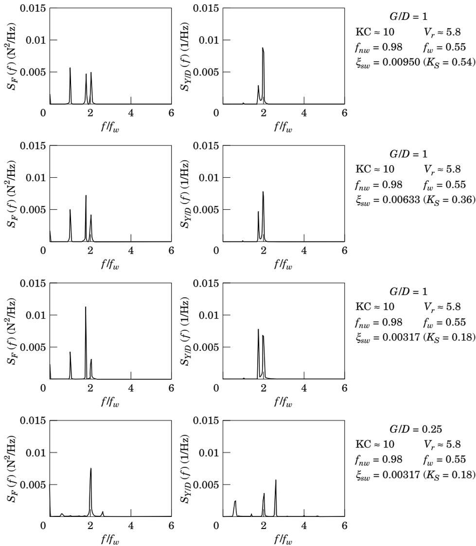
Figure 10. Predicted spectra of wave forces and cylinder transverse responses.
