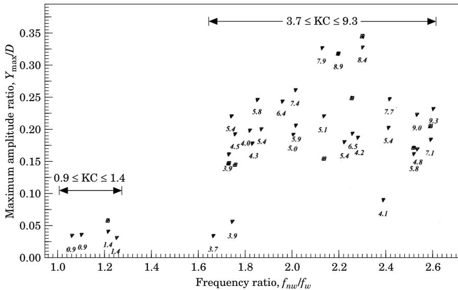
Figure 5. Results of the maximum transverse amplitude versus the frequency ratio  $f_{nw}/f_w$  for various KC numbers;  $D = 0.103$  m,  $G/D = 0.126$  m,  $K_s = 2.73$ . ( $\nabla$ ) Experiments; ( $\square$ ) predictions.
