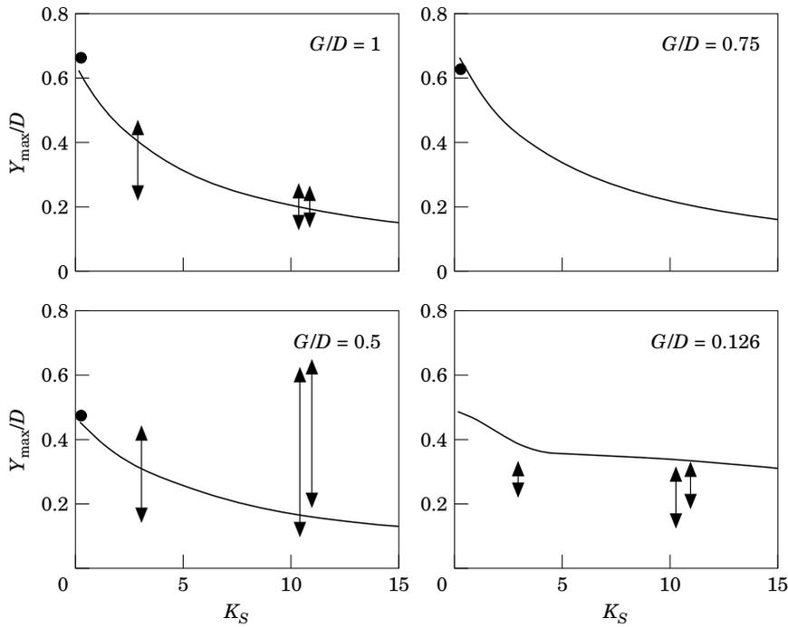
Figure 13. Maximum amplitude of the transverse oscillations as a function of the stability parameter, for  $KC \approx 10$ ,  $V_r \approx 5.8$ ,  $\xi_{sw} = 0.00317-0.2639$ : —, predicted; ( $\bullet$ ) experimental from Anand & Torum (1985); ( $\nabla$ ) present experimental data.
