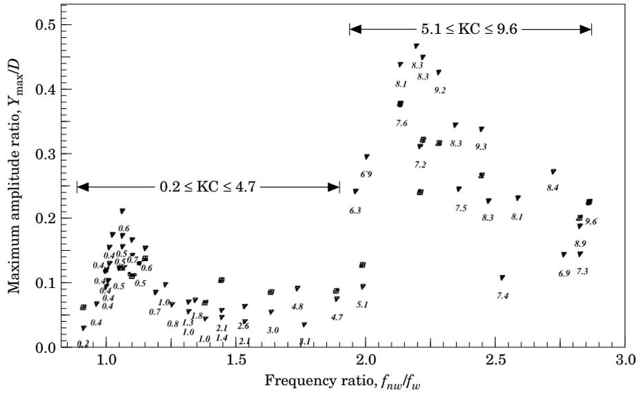
Figure 4. Results of the maximum transverse amplitude versus the frequency ratio  $f_{nw}/f_w$  for various KC numbers;  $D = 0.103$  m,  $G/D = 1$ ,  $K_s = 2.73$ . ( $\nabla$ ) Experiments; ( $\square$ ) predictions.
